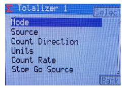
The first option is to choose the mode in which you wish to use the totalizer – completely off or totalizing an analog, frequency, digital or pulse input:
