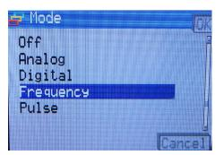
Frequency totalizers or pulse type totalizers are configured automatically within the controller as there is only a single input capable of accepting a frequency or pulse input. However, if you totalize an analog or digital input, an extra screen is displayed where the source for that totalizer is assigned.
