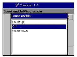
The options presented are **Count up** and **Count down**. In a typical flow application, where the requirement is the total flow through a pipe, you would select the **Count up** option. However for certain applications (such as batching) the option to **Count down** is more appropriate.
