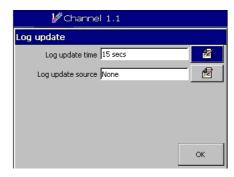
All totalizer events are recorded automatically in the totalizer log. This means whenever you start, stop or reset a totalizer it is recorded along with the value the totalizer has reached at that point. However you also have the option to have the totalizer values entered into the log at regular intervals, either at specified time intervals or by using a digital source.
