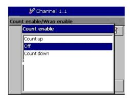
The options presented are 'Count up' and 'Count down'. In a typical flow application, where the requirement is the total flow through a pipe, you would select the 'Count up' option. However for certain applications (such as batching) the option to Count down is more appropriate.
