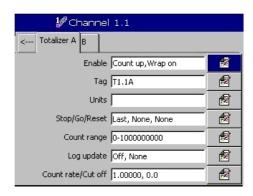
The 'Tag' parameter is a configurable tag used to identify the totalizer in the Totalizer log easily and also to identify the recording channel it refers to.
