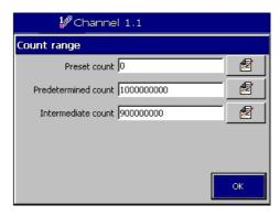
The 'Preset count' is the value at which your totalizer will start counting from – the value applied when the totalizer is reset.
