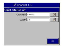
The count rate is determined by the maximum number of engineering units per second and the smallest totalizer increment. For example – to totalize a flow with a maximum rate (Eng High) of 2500 liters / minute (= $2.5 \, \text{m}^3$  / minute) to the nearest 0.1 m³, the calculation Is as follows:
