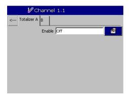
When you first enter the configuration parameter the totalizer is set to 'Off':
