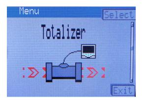
Depending on the functionality available in the CM15, or if you are using the CM30 or CM50, you have up to 2 totalizers available to configure. Select the required totalizer:
