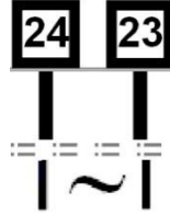
Figure 30. Plug-in Module Slot 2 - Triac Module
