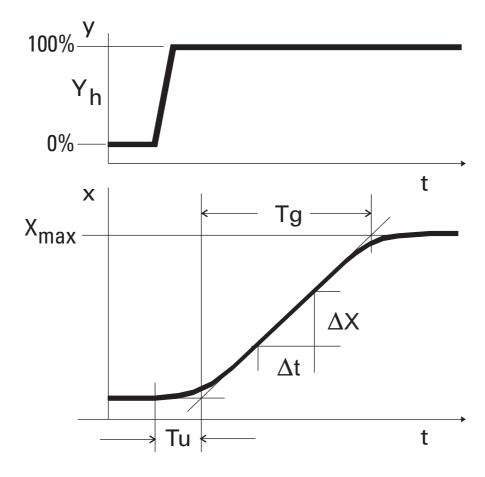
y = correcting variable Y<sub>h</sub> = control range
