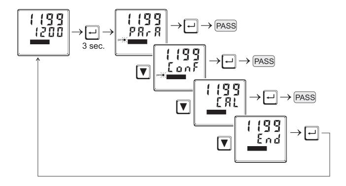
PRrR - level: At PRrR - level, the right decimal point of the bottom display line is *lit continuously*.
