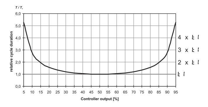
Parameters to be adjusted: **L**: min. cycle time 1 (heating) [s] (PRrR/Entr) **E**?: min. cycle time 2 (cooling) [s]
