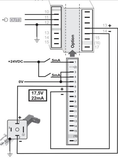
Analog outputs OUT3 or OUT4 and transmitter supply  $U_T$  are connected to different voltage potentials. Therefore, take care not to make an external galvanic connection between OUT3/4 and  $U_T$  with analog outputs!
