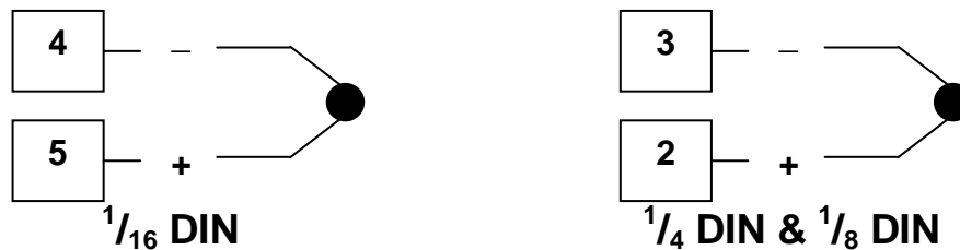
Figure 15. Thermocouple Input Connections
