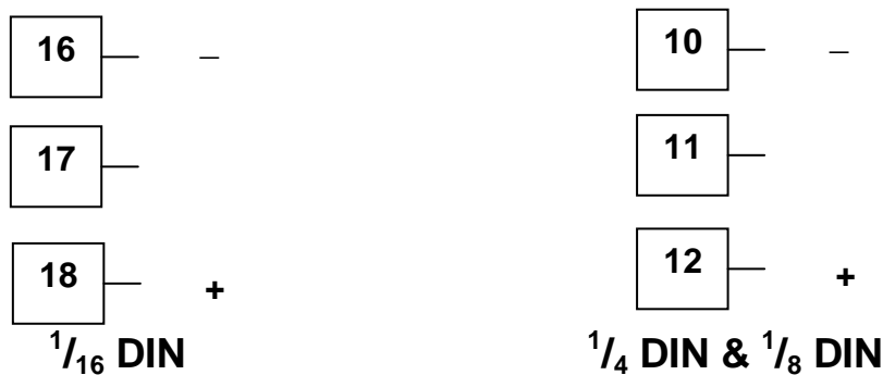
Figure 31. Option Slot 3 - Transmitter Power Supply Module
