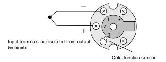
Figure 3 mV input connection.
