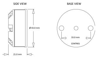
Mounting holes: two holes 5.5 mm diameter, 33 mm centres. Centre hole sensor wire entry 4 mm.
