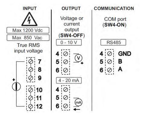
Connect the pole «+» of voltage input, indifferently, to one of the screw terminals 7, 8, 9 (equipotentials).
