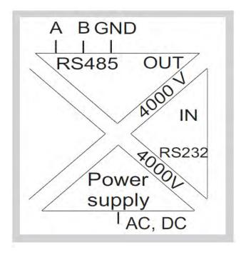
The power supply transformer necessary to supply the module must comply with EN60742 (Isolated transformers and safety transformers requirements). To protect the power supply, it is recommended to install a fuse.
