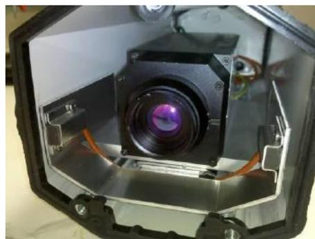
Install front Germanium window cover by tightening 3x screws then install sunshield as shown.
