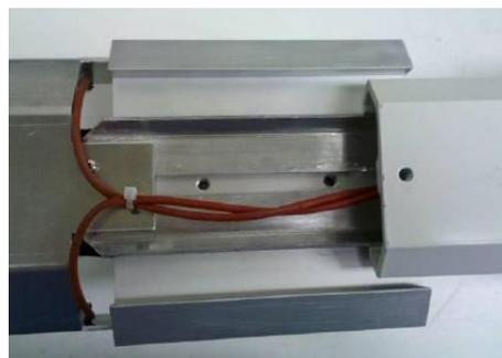
Secure conduction plate to rail by installing 2x Screws (truss), 4x curved washers (2x per screw), and 2x flat washers. Insert each screw half a turn past after making contact with curved washer and slide camera forward.
