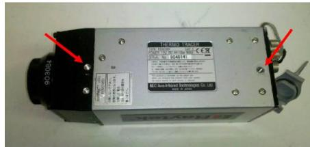
Place conduction plate onto camera as shown, making sure to line up holes on camera with hole and slot on the conduction plate.
