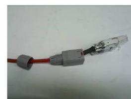
Remove cable from RJ45 jack by lifting tab, note wiring for reassembly.
