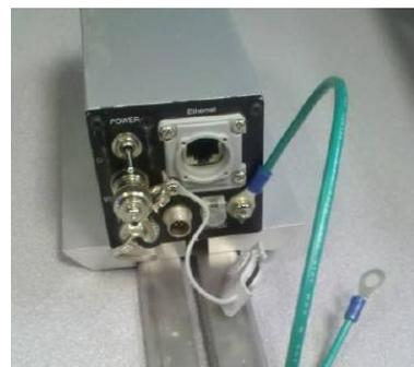
Disassemble Ethernet cable connector by loosening nut as shown.
