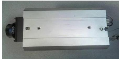
Install 2x M4 screws and secure conduction plate onto camera.
