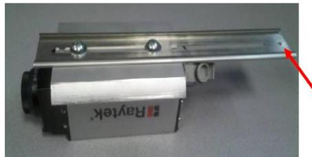
Secure rail to conduction plate by installing 2x screws (truss), 4x curved washers (2x per screw), and 2x flat washers. Insert the screws until each screw makes contact with curved washer; curved washers will be compressed once camera is installed in enclosure.
