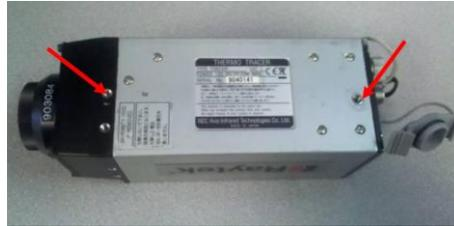
Place conduction plate onto camera as shown, making sure to line up holes on camera with hole and slot on conduction plate.
