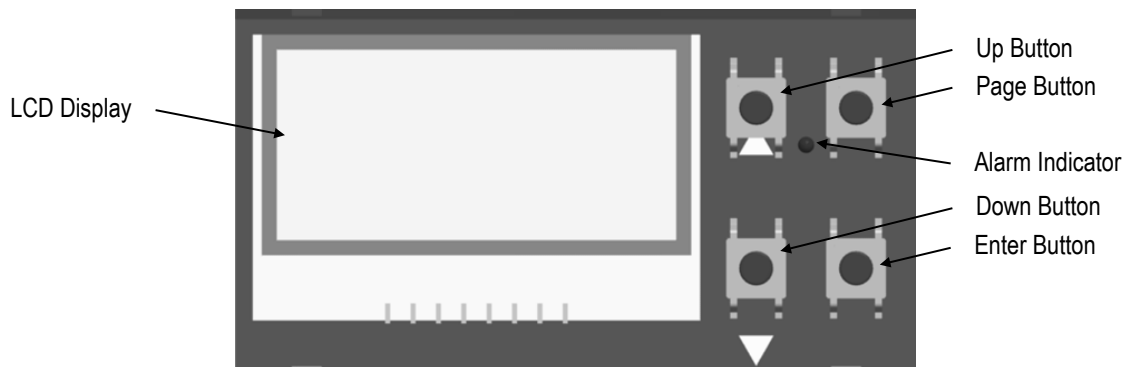
Figure 33: Control Panel for the Comm Box (DIN)
