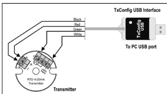
Figure 01 – TxConfig USB Interface connections
