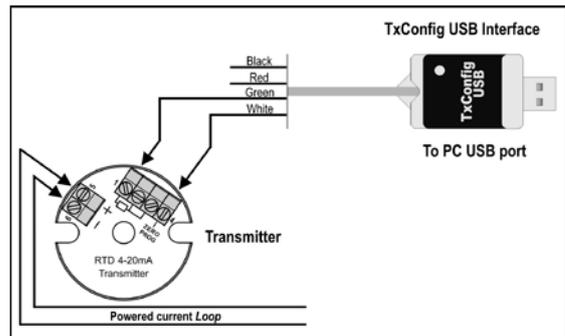
Figure 02 – TxConfig Interface connections – Loop powered
