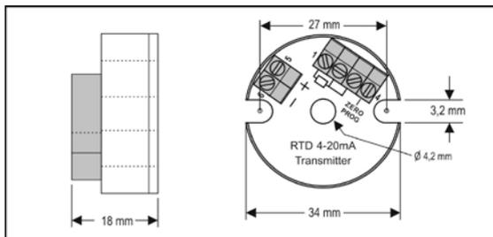
Figure 04 – Transmitter dimensions
