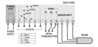
Fig. 2 - N323RHT terminals - Relays share a common terminal (standard model)
