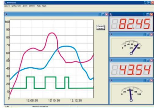
The **myPCLab** software can simultaneously communicate with multiple modules, making easy to expand the number of inputs of a measurement system.
