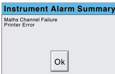
Figure 3.1.4b Typical Instrument alarm summary display
