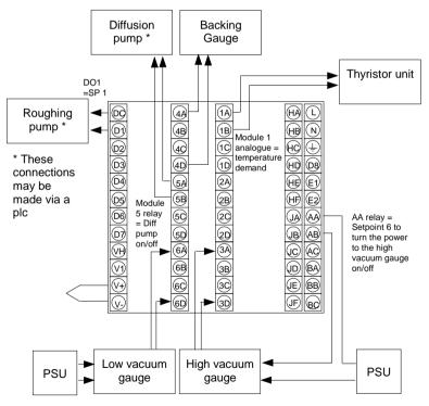
Figure a-4: Example Wiring Connections
