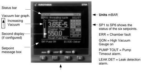
The Loop Select button enables other loop displays, see section 3.4 'Installation and Operation Handbook
