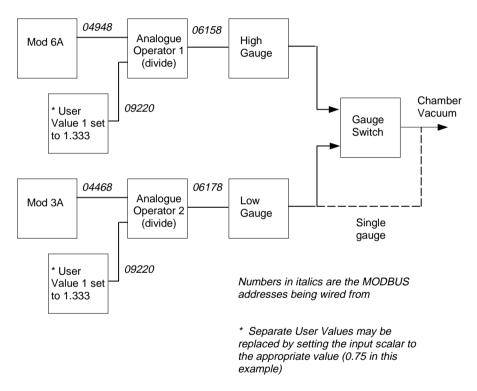
Figure a-8: Scaling units in a two gauge system
