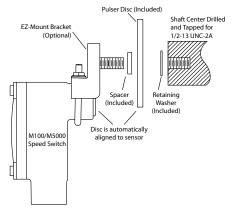
Figure 11: EZ-Mount bracket installation
