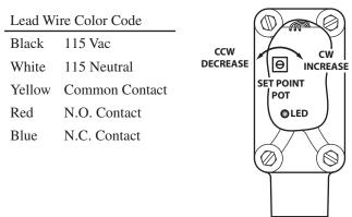
Figure 3: Set Point Adjustment
