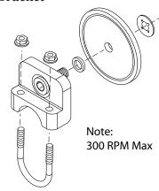
Figure 10: Optional EZ-Mount bracket w/255-EZ Pulser Disc
