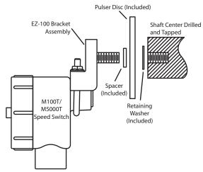
Figure 8: EZ-Mount Bracket installation
