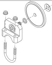
Figure 7: Optional EZ-Mount Bracket w/255-EZ Pulser Disc
