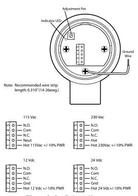
Figure 3: Set Point Adjustment
