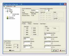
During the configuration process, the Modbus interface of the **DigiGate** will stop working as a master and start operating as a slave. On this condition, a computer equipped with a USB-RS485 is connected to the Modbus interface, and **DigiConfig** software will work as a Modbus network master in order to perform the **DigiGate** configuration.
