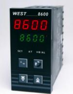
The West 8600 temperature controller can measure and display the heater current. Special heater break alarms give early warning of element failure, to protect equipment and product. A soft-start feature is available for process warm up.
