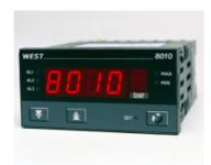
The West 8010 is a 1/8 DIN microprocessor based digital indicator. Available with red or green displays. One latchable relay is fitted as standard, plug-in modules allow two more alarm relays, PV retransmission or transmitter PSU.
