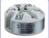
The SEM206/P is a cost effective "smart" in head transmitter that accepts PT100 temperature sensors and converts sensor output over a configured range to a standard industrial (4 to 20) mA transmission signal.
