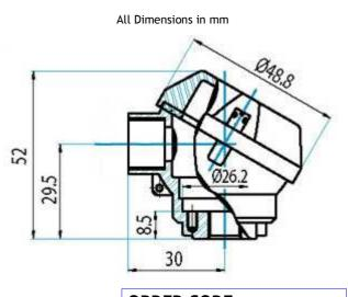
ORDER CODE HTR200V Probe entry M10 x 1.0 HTR201V Probe entry 1/8"BSP
