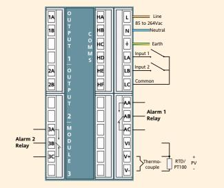
Outputs 1 and 2 are optional outputs which can be any one of the types shown in the tables below. They can be configured for heating, cooling or alarms.
