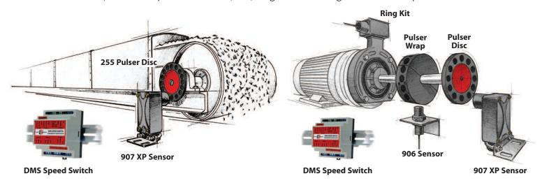
The **DMS-Series** speed switch, designed primarily for OEM use, is the ideal choice for reliable, low-cost shaft speed monitoring on the following types of machinery:
