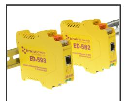
+5 to +30 Volt Power Input enables the device to be run from USB, a vehicle battery or the factory floor
