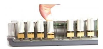
Connect your probes by simply pushing on the terminal top and insert wires of up to 3 mm or 10 AWG diameter and compensated thermocouple connectors.
