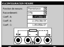
With 50 Kohms range and Steinhart – Hart equation integrated, thermistors can be entered into CALYS 150 and tested. Steinhart-hart equation is as follows:  $\underline{1} = A + B(\ln(R)) + C(\ln(R))3$  T Where: A, B and C are usually calculated according to temperature at 0°C, 25°C and 70°C
