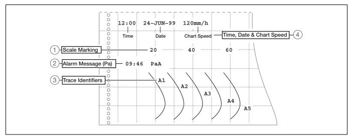
(1) **Scale Marking** – one scale per trace, printed across the width of the zone, at intervals of 20 to 240 mm.
