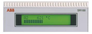
Clear text prompts on the display assist the operator in accessing functions such as chart reload and alarm acknowledge using membrane keys on the front of the recorder.
