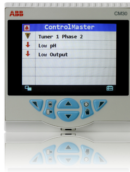
Fig. 3: Alarm status display
