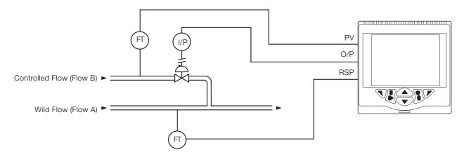
Fig. 21: Ratio controller
