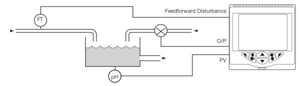
Fig. 18: Single loop with feed-forward
