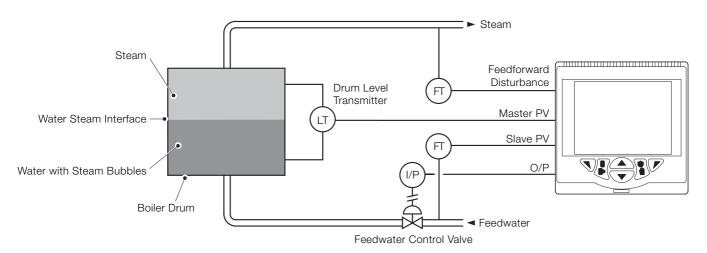
Fig. 20: Cascade with feed-forward
