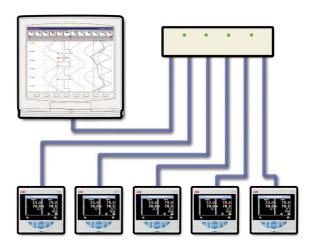
Fig. 14: ControlMasters connected to a ScreenMaster
