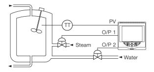
Fig. 10: Split output control example
