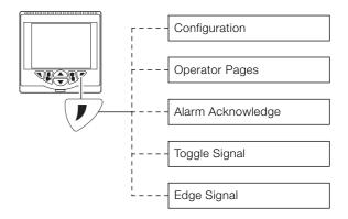
Fig. 6: Programmable soft key
