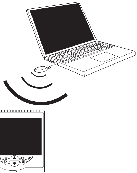
Fig. 16: Transferring a configuration file via the infrared port
