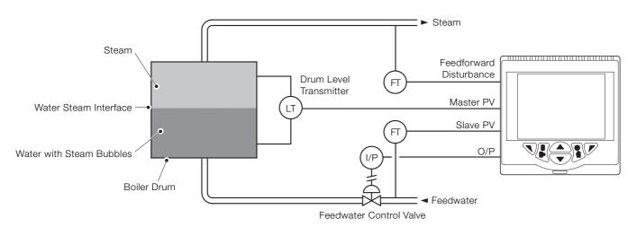
Fig. 20: Cascade with feed-forward
