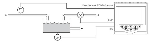
Fig. 18: Single loop with feed-forward
