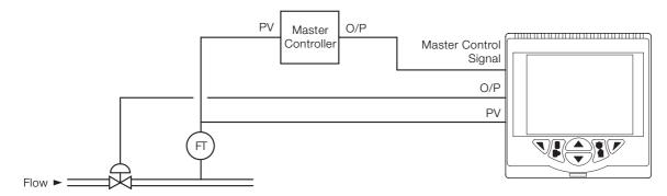
Fig. 23: Auto / Manual station and analog backup station
