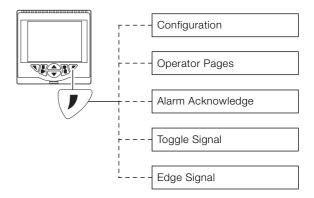
Fig. 6: Programmable soft key
