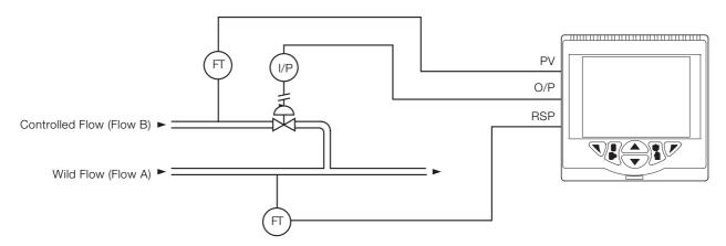
Fig. 21: Ratio controller
