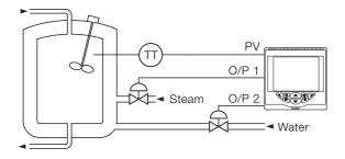
Fig. 10: Split output control example
