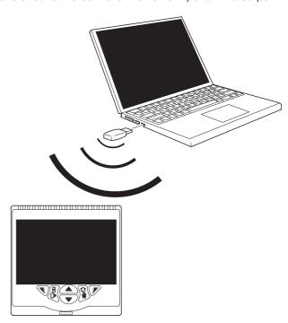
Fig. 16: Transferring a configuration file via the infrared port
