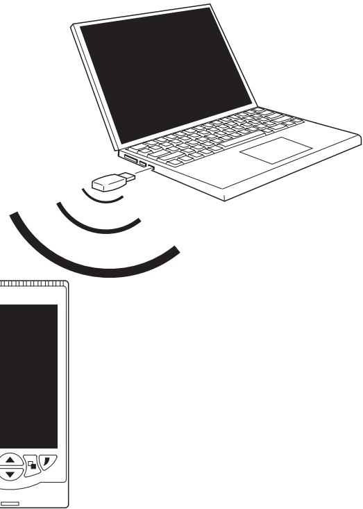
Fig. 16: Transferring a configuration file via the infrared port
