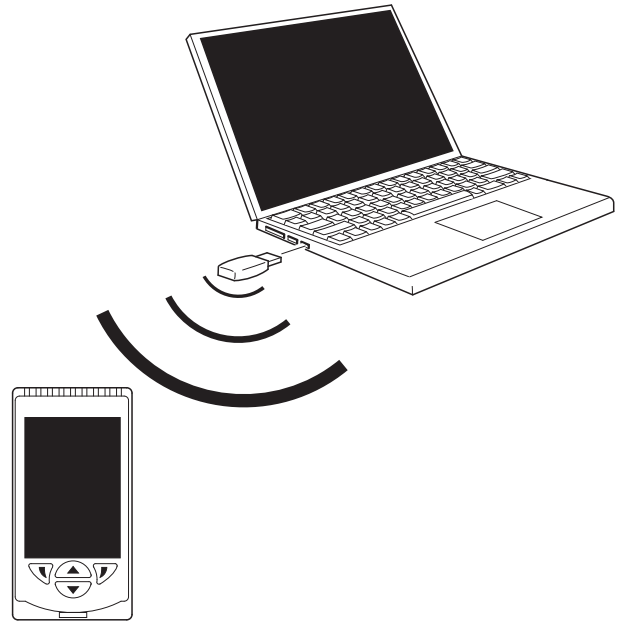
Fig. 13: Transferring a configuration file via the infrared port
