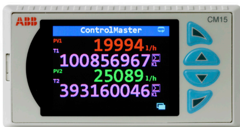
Figure 3 Dual PV and totalization display
